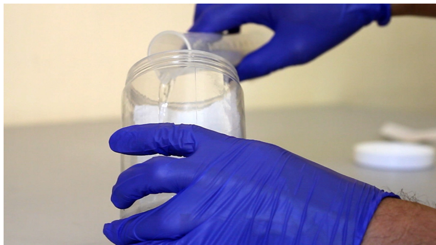
2: Pouring eluent into developing chamber
