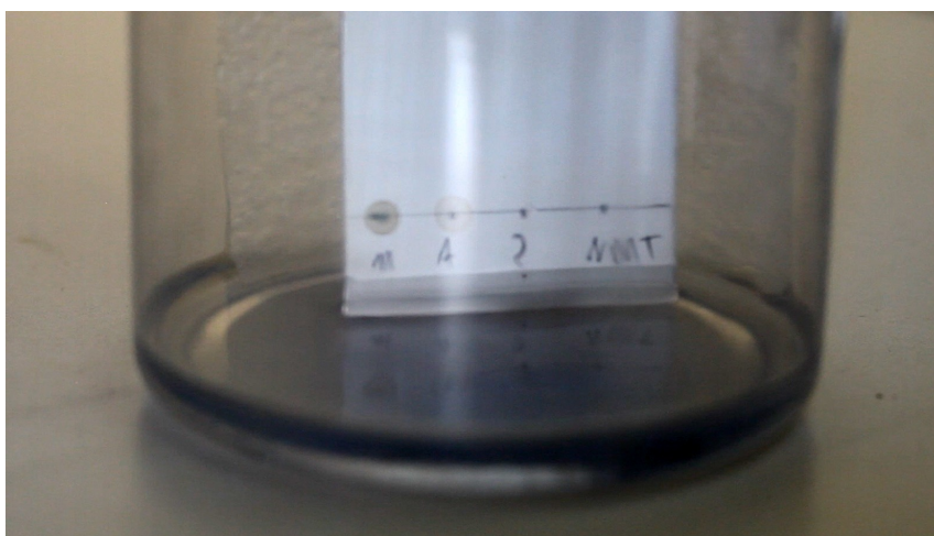
5 Plate starting to run and soak up the eluent
